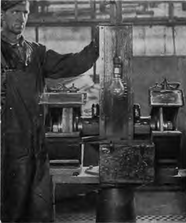
Fig. 1. Hoods, Belt Guard, Plate-Glass Eye Shields, etc., for Emery Wheels.*
